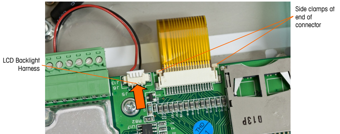
Figure 5-12: Display Harness Removal
