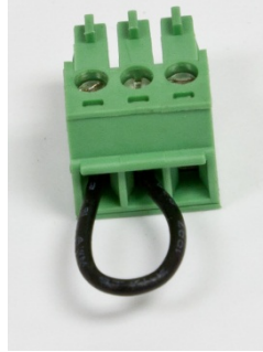
Figure 5-6: Jumper Wire Between COM1 Transmit and Receive Terminals
