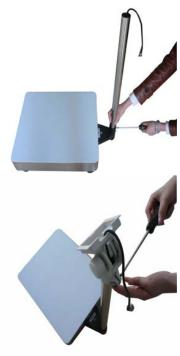
Note: if the load cell connector is too big to thread through the bracket, separate the Bracket by Removing the Knob pole (7), see the following pictures.
